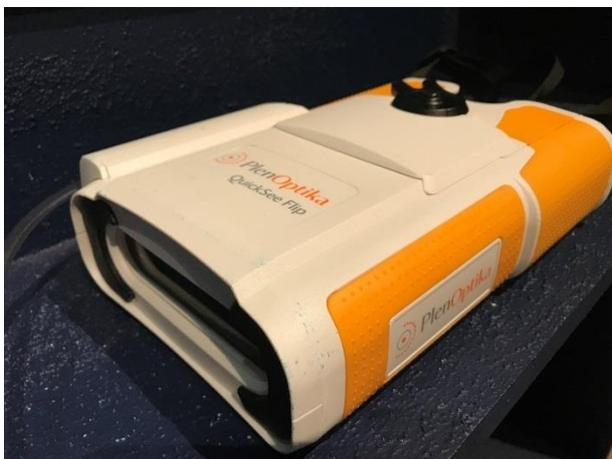
Quicksee is a portable device that allows healthcare workers with no optometry training to deliver accurate eye tests. In developing countries there is often limited access to specialised eye care and the expensive equipment it requires, meaning that people are unable to obtain prescription eyeglasses. This drastically affects their quality of life, educational potential and job opportunities. Quicksee is easy to use and displays a prescription estimate within approximately ten seconds.
